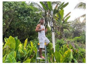
The agent also installed the ATMOS soil probe and system (in partnership with Palau Community College at a taro patch in Laura Village. The ATMOS system collects meteorological, groundwater, Electrical Conductivity (EC), and soil water content data every two weeks and these climate data are used as early warning systems.
